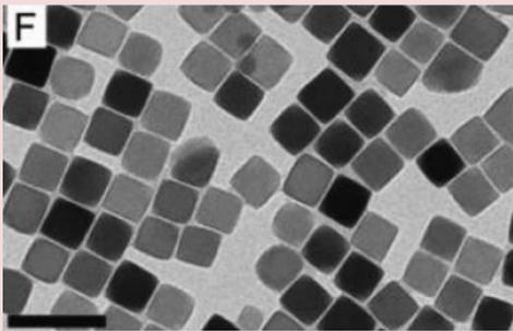
Figure 1: TEM samples of iron oxide nanocubes from reference [3]
