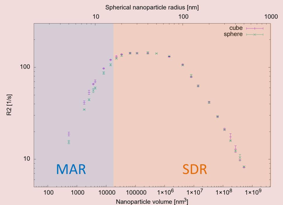
Figure 3: simulation results for spherical and cubic nanoparticles. Abscissa are expressed in volume units for both shapes and in radius units for the sphere case.
