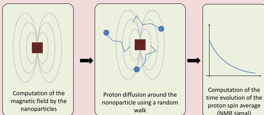
Figure 2 : the three main steps of the simulation of the NMR relaxation induced by IONP
